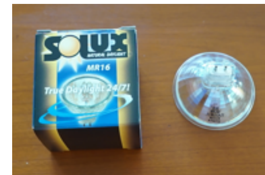
High temperature halogen lamp (4700 K) for calibration
