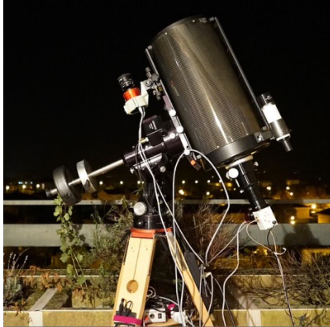
All mirror telescope (GSO 254 mm f/8) Optimal UV transmission and no chromatism
